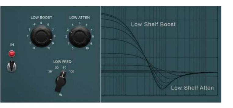
The Pultec EQP-1A low-frequency section shown with its response curves and resonant shapes.
