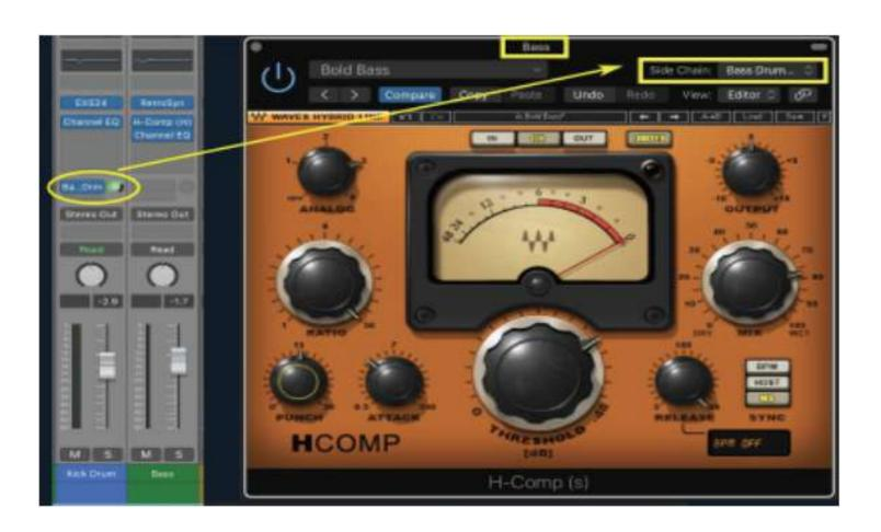
Here we can see the Bass Drum track is sending signal into the sidechain of the Waves H-Comp, which is compressing the Bass track. The Sidechain section selects which aux bus triggers the compressor.
