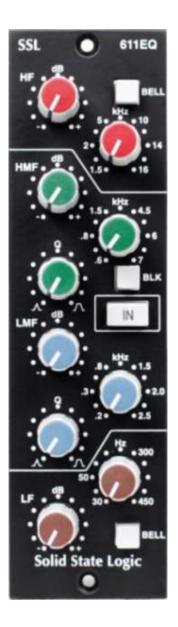
With dedicated controls for frequency, gain, and bandwidth, sometimes called Q, parametric EQs offer more flexibility than graphic or selectable equalizers. Analog parametric EQs typically range from three to eight bands, while digital parametric EQs may offer even more bands. (See SSL 611E parametric EQ pictured here)
