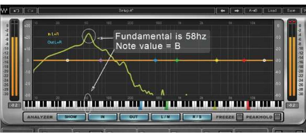
The Waves H EQ provides a spectrum analyzer that overlays the frequency response on top of the equalizer settings.
