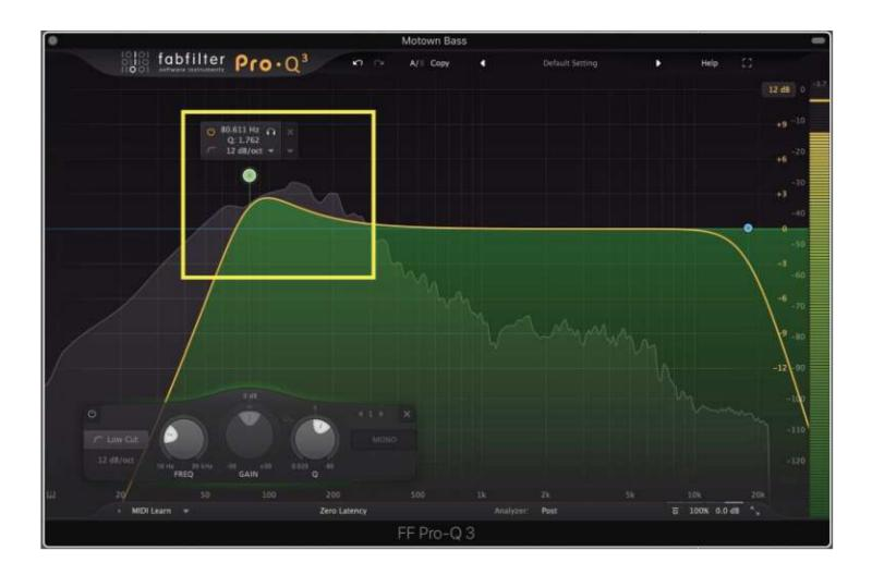
The versatile FabFilter Pro-Q3 can create a high-pass filter with a resonant boost at the cutoff frequency. This shape can boost the fundamental frequency while cleaning up the muddy subs. You can also see the frequency analyzer displayed behind the EQ curve.
